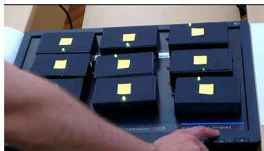
(d) Upon a successful initialization all the devices should turn their green LED ON.
