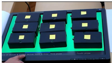
(b) The screen detects all devices and the user initiates the association procedure by clicking on the button shown at the bottom of the screen.
